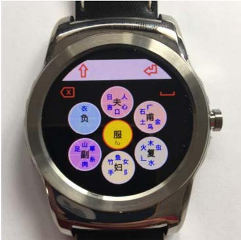
Fig.1 – The iBeezi® keyboard running on an LG Watch Urbane. with typing (dot).
