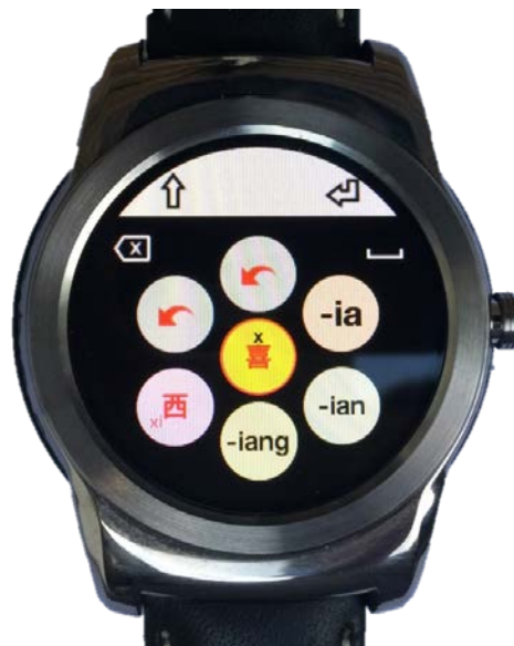
Fig.4 - Second step on the dynamic virtual iBeezi ® keyboard: selecting the final Pinyin component
