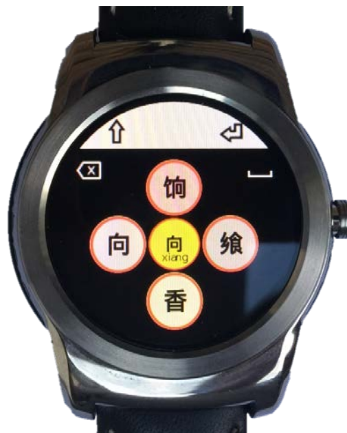
Fig.6 - Fourth step (final Chinese character selection) on the dynamic virtual iBeezi® keyboard
