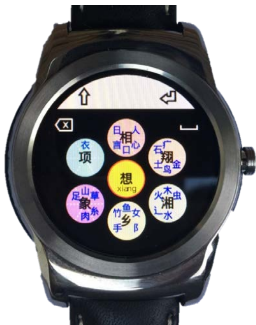
Fig.5 - Third step (Radical selection) on the dynamic virtual iBeezi® keyboard: selecting the Chinese radical associated with the character
