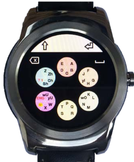
Fig.2 – The iBeezi ® keyboard running on an Android Wear (LG Urbane watch)
