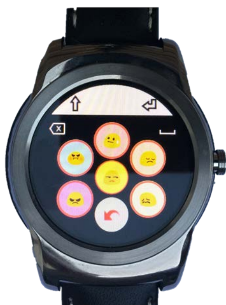
Fig.7 - Selection of emojis on the dynamic virtual iBeezi® keyboard
