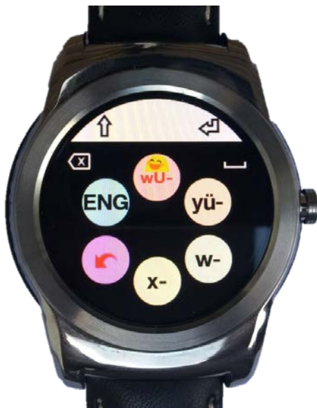
Fig.3 - Starting screen of the six-key dynamic virtual iBeezi ® keyboard: encoding a Chinese character starts, as a first step , with selecting its initial Pinyin component
